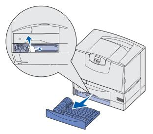
2 Reinstall the duplex mechanism in the printer.
